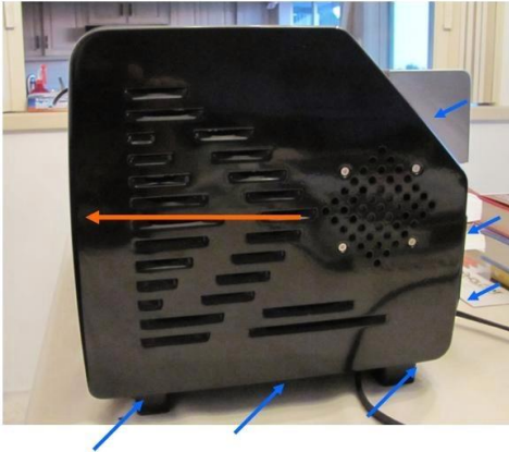
Remove 6 screws (blue arrows), slide panel forward (orange arrow) set panel aside
